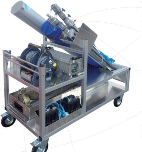
Thanks to their aluminum rim with solid rubber tires, the wheels have hardly any rolling resistance and, despite the weight, guarantee easy mobility of the car even in rough terrain. The independent wheel load is 400 kg.
