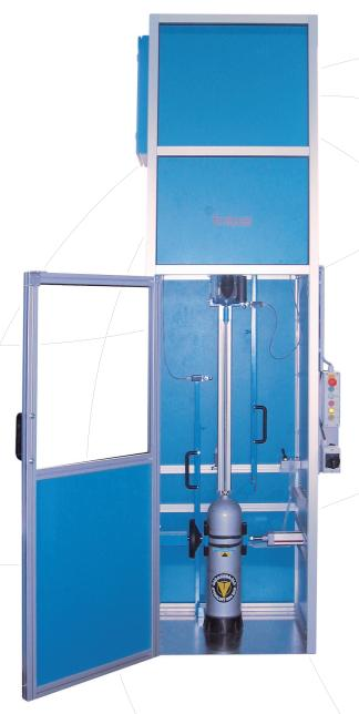
The rotation of the cleaning brush controlled by frequency converter is approximately 1450 rpm. Therefore we guarantee, that the inside of the steel cylinder will be cleaned completely from rusty deposits.
